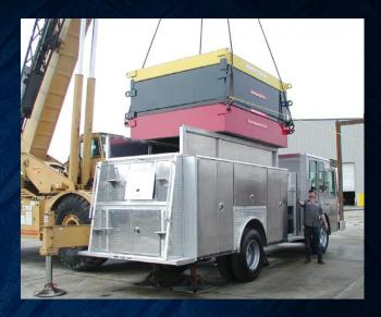
We don't just say we have the strongest trucks in the industry; we back it up by putting them to the test. Our custom body is tested against regulation 29 (ECE R29) and exceeds all test requirements. We went a step further by placing 66,000 lbs. on top of the body, which showed no structural deformity and demonstrated the impressive strength of Ferrara fire truck bodies.
