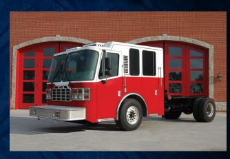
To protect the protectors, Ferrara cabs are designed with heavy-duty components and construction. We build our cabs with extruded aluminum roll cage framework in the roof, sidewalls, doorjambs and floor. Marine grade aluminum, the thickest and strongest used in fire cab construction, is used throughout the cab.
